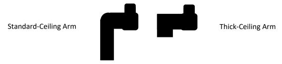
The standard mounting arms of the RSL C34E accommodate ceilings with a maximum thickness of 3/4 inch. For ceilings with a thickness (up to 2 inches), replace the standard mounting arms with the shorter ones that are included with your speaker.
