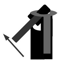
**Step 3:** Twist the mounting arm in the direction shown until it clears and you can remove it.
