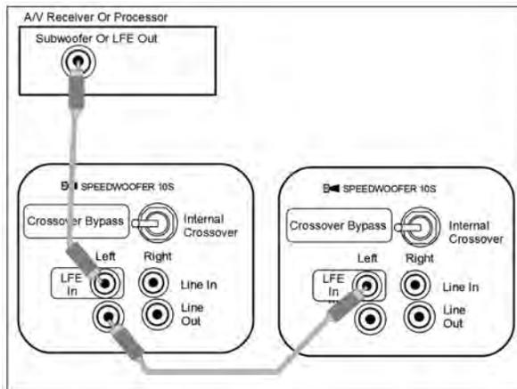
**Connecting Two Subs - A/V Receiver Or Processor**
