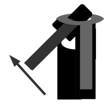
**Step 3:** Twist the mounting arm in the direction shown until it clears and you can remove it.
