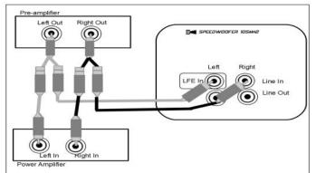
Method #2 - Connection Using Y Adapters
