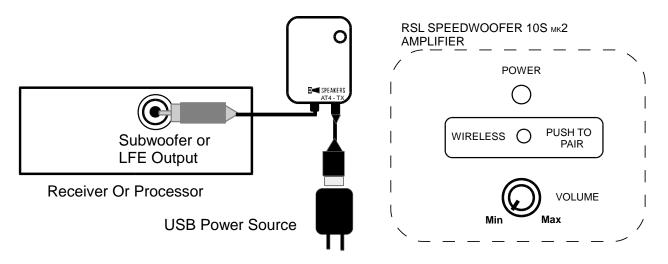
The optional RSL AT4 wireless transmitter lets you send audio wirelessly to a receiver built-in to the Speedwoofer 10SMKII. A wireless connection can be handy when it's difficult to run an RCA cable to your subwoofer.
