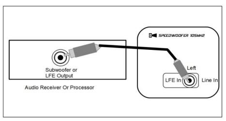
**Connection to A/V Receiver Or Processor**
