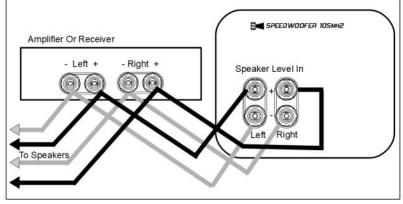
Method #3 - Connection Using Speaker Wires
